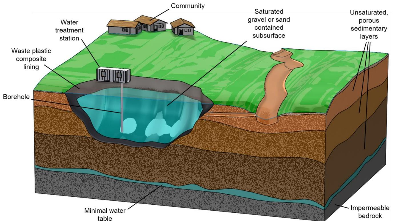
Figure 1: Dry season- showing the aquifer construction and water retention during dry season.
